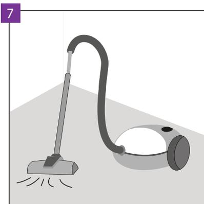
Make sure that the substrate is dry, flat, stable and free of any grease or chemical substances. The protruding irregularities must be scratched off and removed. Before the installation, the ground must be swept and vacuumed carefully so as to remove any contamination. It is necessary to repair any more serious imperfections of the substrate and large cracks.
