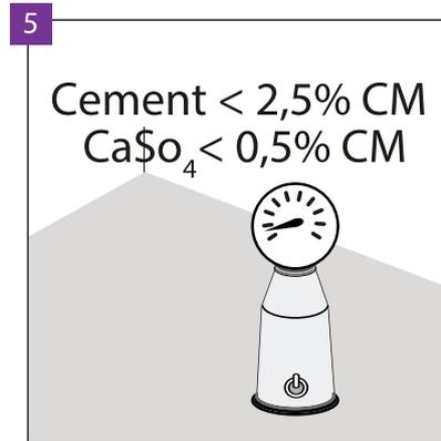
In the case of the cement grout, the moisture content in the substrate must be lower than 2.5%, and in the case of the anhydrite grout, it must be lower than 1.5%. In the case of installation with the underfloor heating, the above-mentioned values must be 1.5% and 0.3% respectively.
