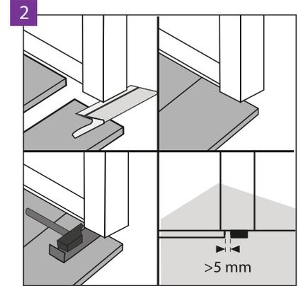
Expansion joints along the walls must be covered with a decorative strip, assembling it by means of glue or special clips. It is recommended to use the Arbiton strips dedicated to a given panel, which guarantee the excellent colour match and the coat resistant to scratching.
