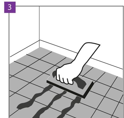
In the case of installation on the substrate covered with ceramic tiles, fill the tile joints with the gap wider than 4 mm and deeper than 1 mm with a durable compound for the filling of points, e.g. resin grout. Installation is allowed on tiles with grouts not wider than 5 mm and 1 mm deep without using levelling compound, provided the Multiprotect Hardlay or Vinclic Solid are used as underlay.
