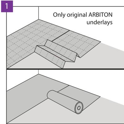
Lay the Arbiton underlay: Multiprotect LVT or Secura LVT Click Smart N perpendicularly to the direction in which panels are laid. The neighbouring ribbons of underlay must be fit tightly and joined by means of an overlap or Arbiton AluTape, without leaving any redundant space.
